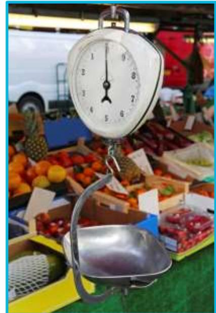
Most spring scales are marked "Not Legal for Trade" in large letters because the accuracy is really an approximation. Also, the spring in a spring scale can permanently stretch with repeated use and so will become even less accurate over time.
