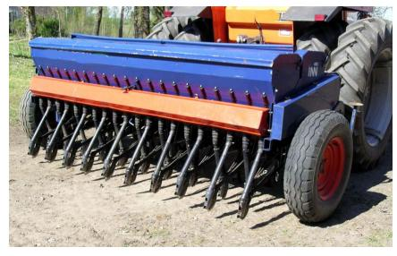
seeded by throwing the seeds over the field, sometimes called "manual broadcasting." Some seeds landed in the furrow and were protected, which others might be left exposed...not very efficient! The use of a seed drill can boost the ratio of crop yield by up to nine times, by placing seeds just where they are needed.
