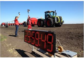
The Maestro 24.70 SW single-grain seed drill manufactured by Horsch drills 24 seed rows with a spacing of 70 cm and a sowing depth of between 1.5 and 9.0 cm. For the world record attempt, the depth was set to 6 cm. The seeds are fed by a "Seed on Demand" system, which ensures easy filling and shortens filling times. The central tank has a seed and fertiliser capacity of 2,000 litres and 7,000 litres respectively.
