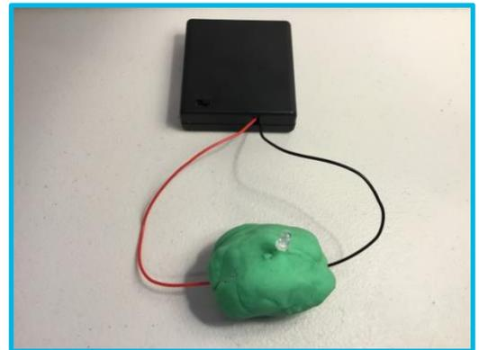
2. Next, separate the conductive dough into two pieces. Insert one battery pack wire into one piece of dough and the other into the other piece of dough. Now insert the LED with one lead in one piece of the dough and the other lead in the second piece of dough. What happens?
