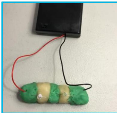
**Parallel circuits** allow multiple paths for electricity to flow through. In a parallel circuit with LEDs, each LED has electricity flowing directly to it along its own path. Each LED can shine brightly no matter where it is, because the electricity is reaching each LED directly. Also, in a parallel circuit, if one light burns out or is removed, the others will continue to shine.
