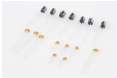
Electrolytic capacitors (top), ceramic capacitors (bottom).
