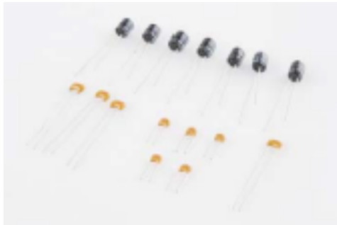
Electrolytic capacitors (top), ceramic capacitors (bottom).
