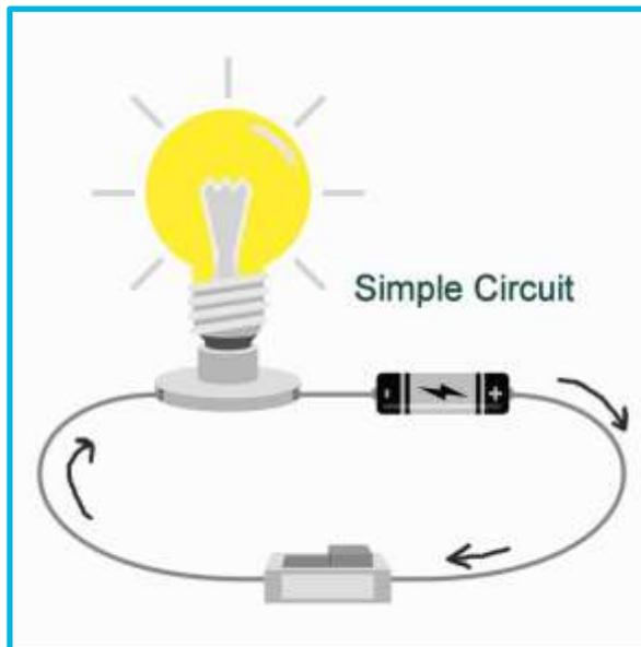
◆ **Schematic Diagram of a Simple Circuit**
