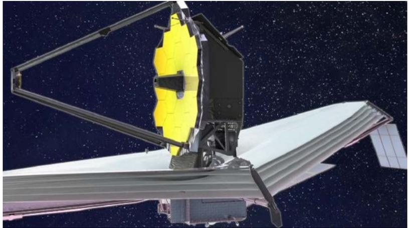
Once the Webb telescope is on its way to its final orbit, approximately 1 million miles from the Earth, engineers at Northrop Grumman will issue commands to the Webb Telescope to unfold it. "Think of the sunshield as five candy wrappers the size of a tennis court," said Mark Clampin, Webb Telescope Observatory Project Scientist at NASA's Goddard Space Flight Center, Greenbelt, Maryland.
