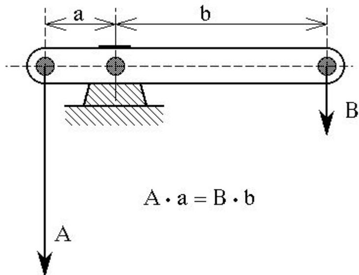
Wheel and axle: A wheel is essentially a lever with one arm the distance between the axle and the outer point of the wheel, and the other the radius of the axle. Typically this is a fairly large difference, leading to a proportionately large mechanical advantage. This allows even simple wheels with wooden axles running in wooden blocks to still turn freely, because their friction is overwhelmed by the rotational force of the wheel multiplied by the mechanical advantage.
