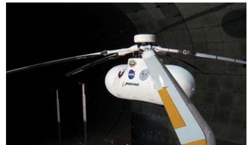
NASA tested this rotor design in a wind tunnel to research ways to make helicopters quieter. Image Credit: NASA
